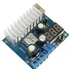
DC-DC Boost Converter CC CV 3...35V
