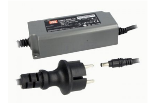
Nättaggregat: switchat; Mean Well OWA-60E-24, 60W; 24VDC; 0...2.5A, IP67
