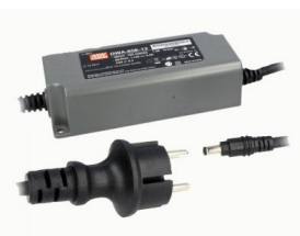
Nättaggregat: switchat; Mean Well OWA-60E-54 60W; 54VDC; 1.12A, IP67
