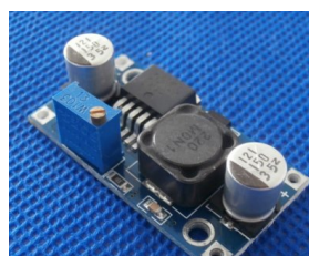
DC/DC Boost Converter 3.5-32V Step-up to 6-35V 3A
