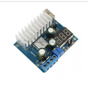
DC-DC Boost Converter CC CV 3...35V
