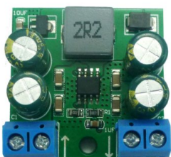
DC-DC Step-Up Boost Converter Module, 5V 3A
