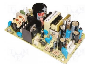
Nätaggregat Mean Well +5V 2A +24V 1A PD-25BNO
